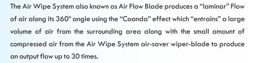
Air Wipe - Circular Air Knife blow off, clean, cool and dry cables, pipes, extrusions, hoses, wires and ropes. Air Wipe - Circular Air Knife is easy to mount and maintain and reduces both compressed air consumption and noise levels. Air Wipe - Circular Air Knife is available in aluminum or stainless steel 316L.
